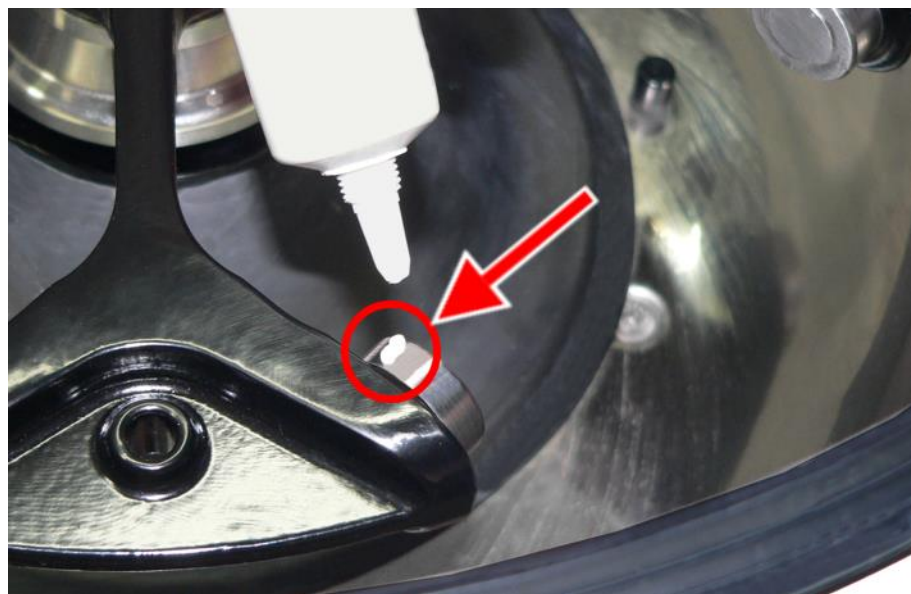
Fig. 29: Sufficient quantity of grease for one bolt
