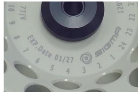
Fig. 4: Different service life – engraving on the bucket/rotor
