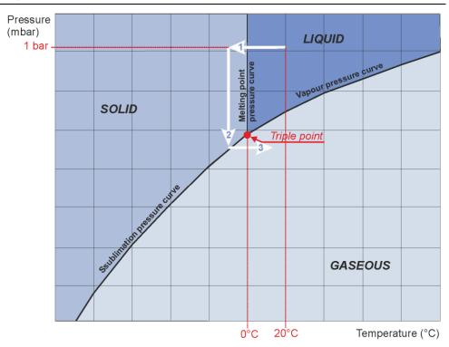
Fig. 8: Freeze-drying phases
