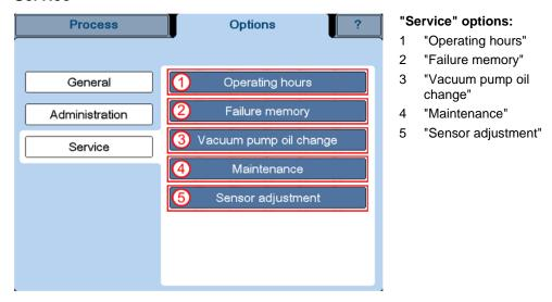
Fig. 43: Dialogue box "Service" (varies depending on the type of freeze-dryer)
