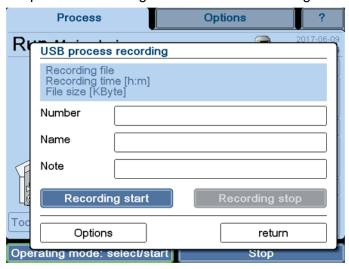
Fig. 23: Dialogue box "USB process recording"
