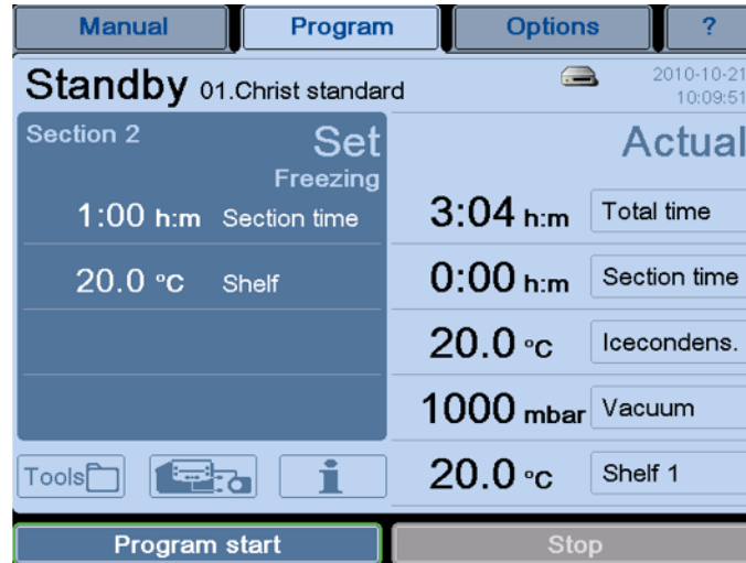
Fig. 73: The freeze-drying process can be started with the aid of the button "Program start".
