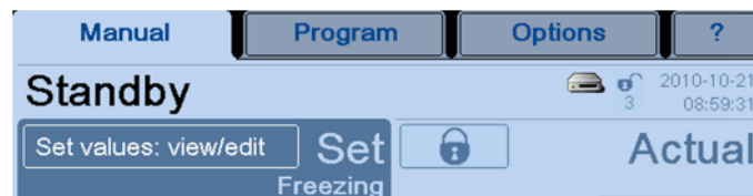
Fig. 46: Countdown of the password timer and the button with the lock symbol
