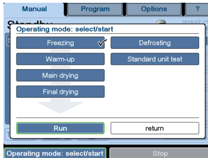
Fig. 31: Dialog box "Operating mode: select/start" (The version of the dialog box that is displayed depends on the equipment of the freeze-dryer.)
