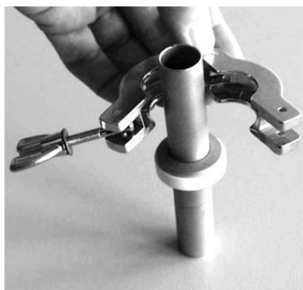
Fig. 76: Attaching the clamping ring
